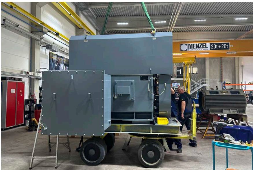
Caption: Menzel configured a squirrel cage motor from stock for use in zone 22 hazardous areas with potentially explosive dust atmospheres and for converter operation, designing it for an efficient smooth replacement in the customer's plant
