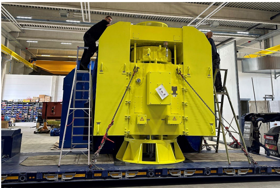
Caption: The vertical motor also supports the weight of the driven pump and therefore features an especially robust design
