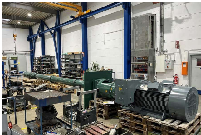
Caption: Menzel supplied complete pump systems with drive and connection pipes from a single source
