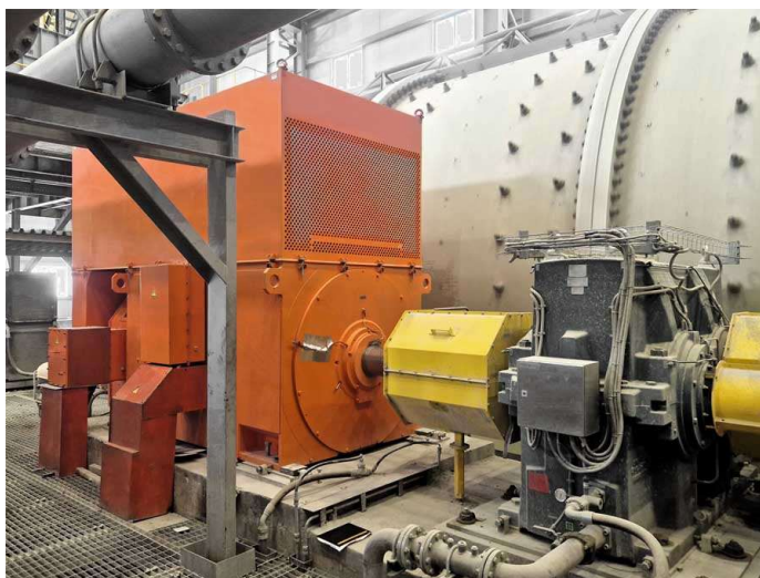
Caption: Alchemist secret revealed – this is how to make gold from iron and copper: a pair of heavy-duty motors propel the ball mill of a gold mine
