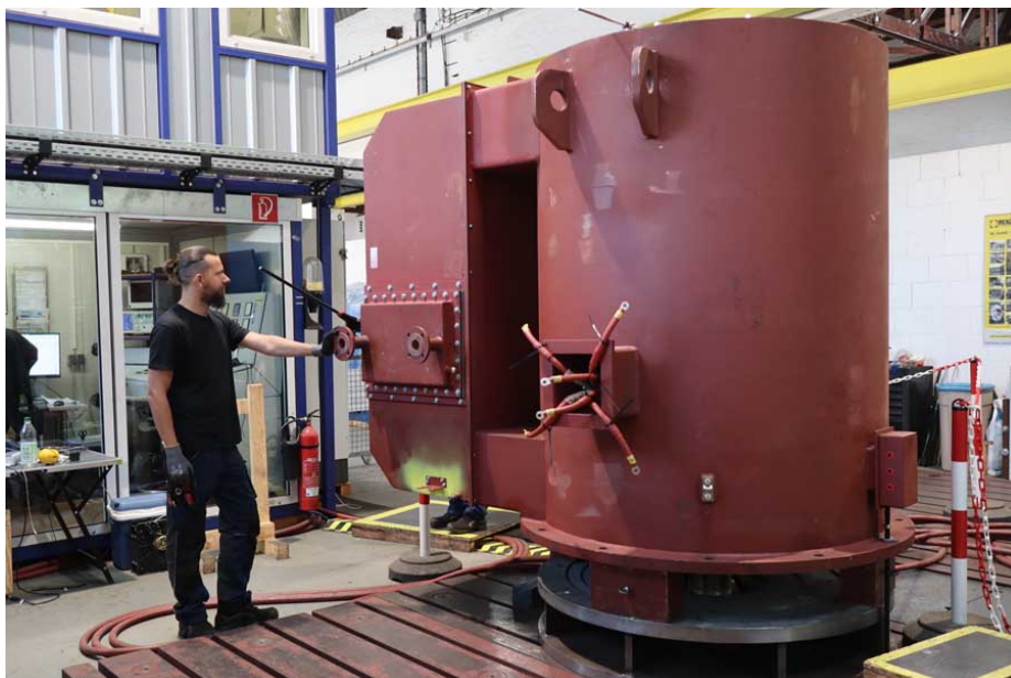
Caption: The special motor can drive a ship's azimuth thruster at two different speeds thanks to two separate windings
